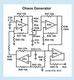
It is a circuit that will produce a chaotic signal output and also a wide variety of multiply periodic signals. It consists of three standard single-opamp oscillators connected in a ring. The Shape control varies the signal's waveform. When tuned to a chaotic regime, the signal acts much the same as a noise source in a S/H application. When tuned into other waveforms, the sampled output is more correlated in time.
