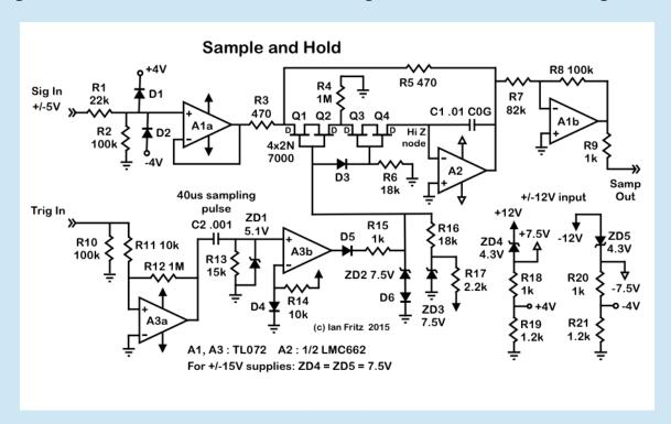
The circuit operates from +/-12 V supplies. ZD4/ZD5, R18/20 and R19/R21 provide +/-7.5 V and +/-4 V subregulated voltages for the CMOS opamp supply and the input clamp, respectively. These should be bypassed with capacitors to ground (not shown). Input signal levels should be in the +/-5 V range.
